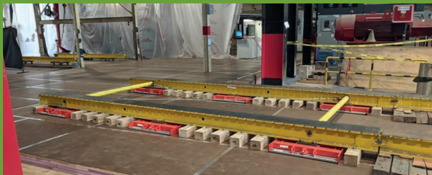
A skidding system was combined with air-skates on a lightweight “dance floor.”
