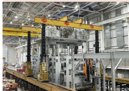
DHGC installed a five-stand press line in a shallow 5-meter-deep pit.
