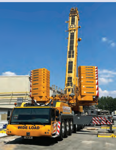
The Liebherr LTM 1450-8.1 offers a max capacity of 550 tons and max radius of 335 feet.
