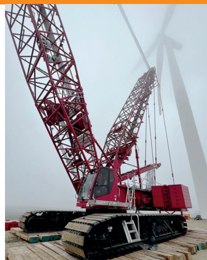
Nordic Crane’s new Tadano CC 38.650-1 lattice boom crawler crane at work in Norway
