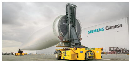
The other end of the new load carrier with an adaptor to carry a turbine blade
