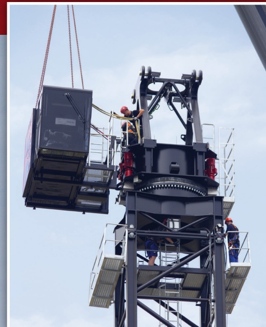
Enlarged cabin unit with enclosed electric cabinet in the colours of the first customer. Access to the spacious cabin is provided by a platform which can be used for emergency treatment of the driver
