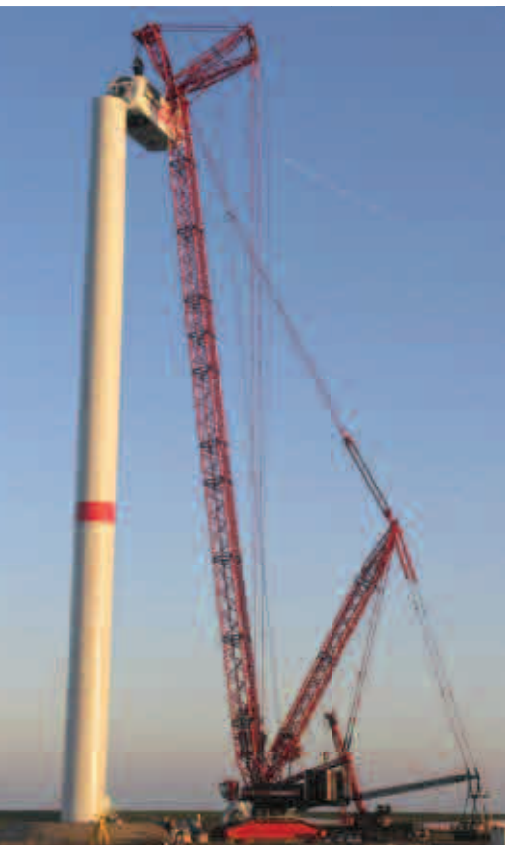
Liebherr's flagship, the LR 11350 is a 1,350 metric ton (1,500 ton) capacity crawler crane
