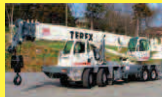
75T TEREX T 775 Truck Crane
