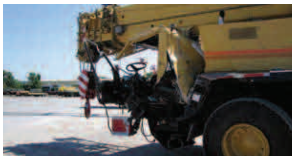
Before: Grove GMK5130 with a damaged cab.
