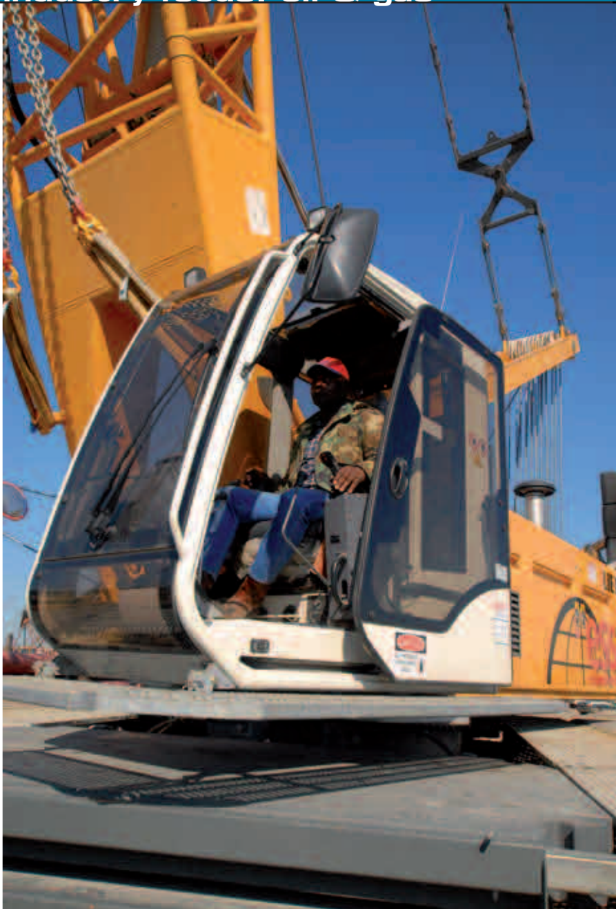
Above: Macarthur “Mac” Carvin operates the 463,000 pound, 275 ton capacity Liebherr LR 1200 SX, carefully loading the specialized pipe for the pipeline of the Atlantis deepwater oil and gas field in the Gulf of Mexico
