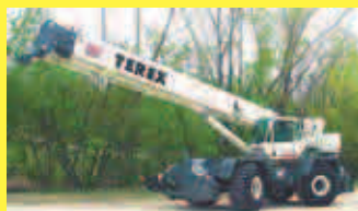
65T TEREX RT 665 Rough Terrain Crane
