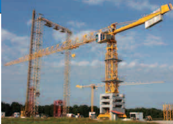
Potain's new MDT 218 flat top tower crane with distinctive counterjib
