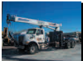
Manitex 2281 Unit #: MX050022 22 ton 81' main boom Tractor mount package 2006 Sterling LT7501 300HP Cat Engine $170,000
