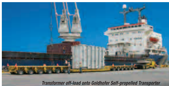
Transformer off-load onto Goldhofer Self-propelled Transporter
