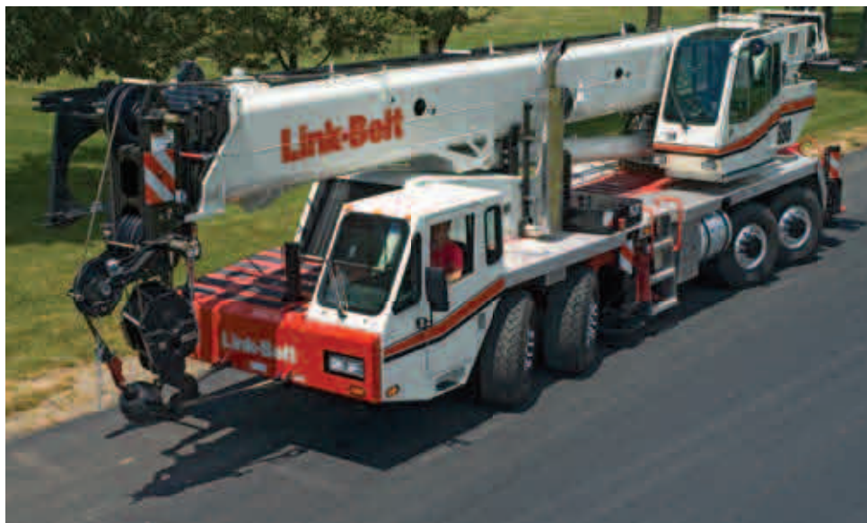
Link-Belt's 90 ton HTT8690 hydraulic telescopic four axle truck crane
