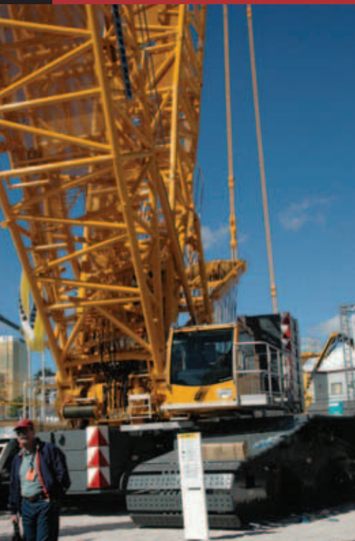
ABOVE: Known for its performance on US wind farms, the 660-ton Liebherr LR 1600/2 crawler can be rigged with a 617-foot boom, with a 315-foot main boom and a 315-foot luffing jib
