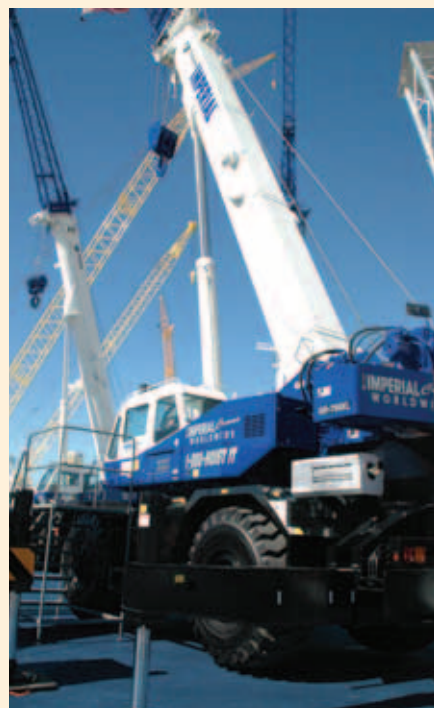
ABOVE: The Tadano 75-ton GR 750XL rough terrain crane is among several ATs, truck cranes and boom trucks at the tadano booth
