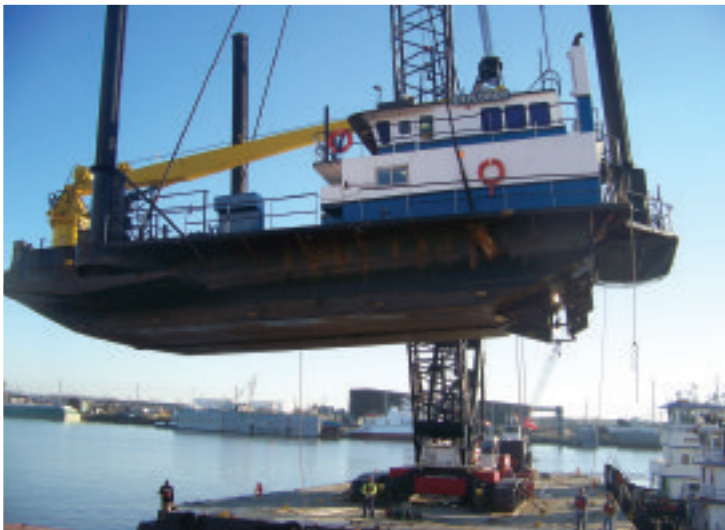
Big Al launches a small jack up boat at the Port of Mobile. The crane is lashed to a 212 foot by 68 foot barge
