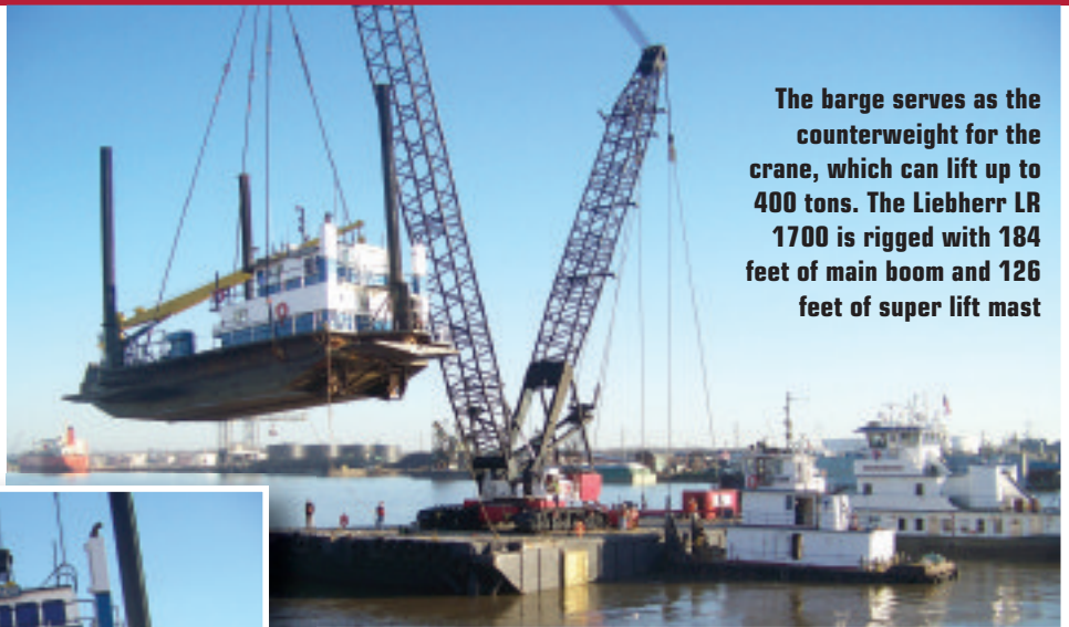
Big Al launches a small jack up boat at the Port of Mobile. The crane is lashed to a 212 foot by 68 foot barge
