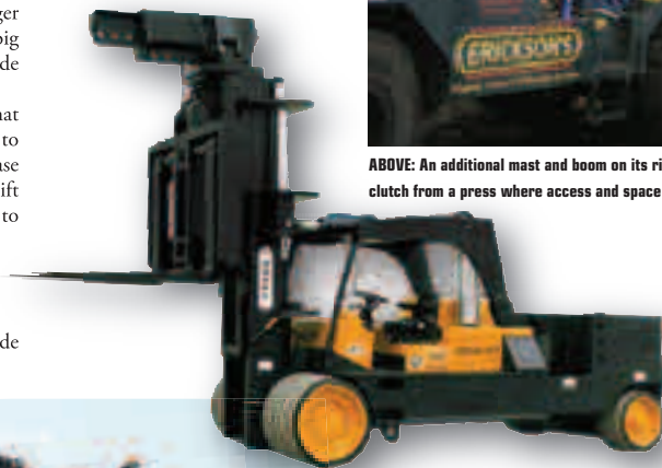
ABOVE: Royal, based in New Century, KS, manufactures a range of specialized rigger trucks. The 80/100 model pictured has a capacity of 80,000 pounds retracted and 100,000 pounds extended at 36 inches
