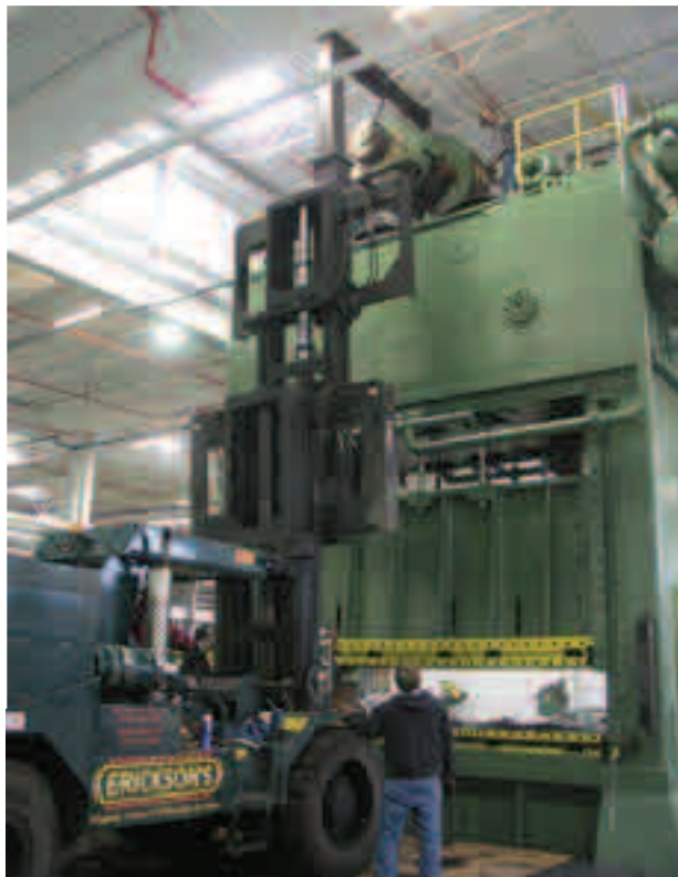
ABOVE: An additional mast and boom on its rigger truck allowed Erickson's to remove a clutch from a press where access and space was very limited
