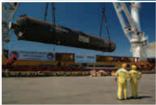
The 628 ton reactor being unloaded by Big Lift's Happy River on to Dock 16 in the Port of Houston
