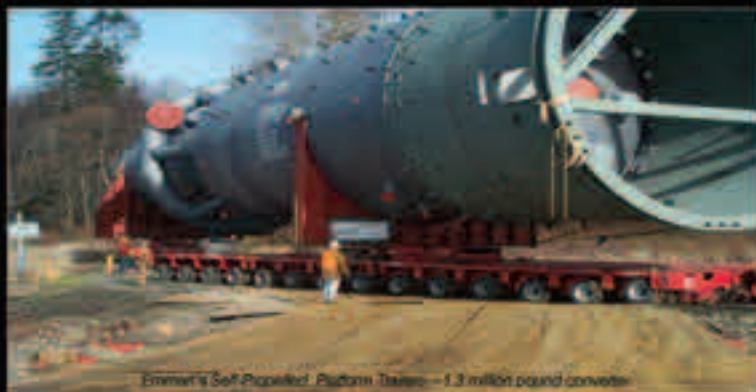
Emmert's Self-Propelled Platform Trailer—1.3 million pound converter
