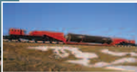
ABOVE: The reactor suspended between the Schnabels, or arms, of the 36 axle rail car combination
