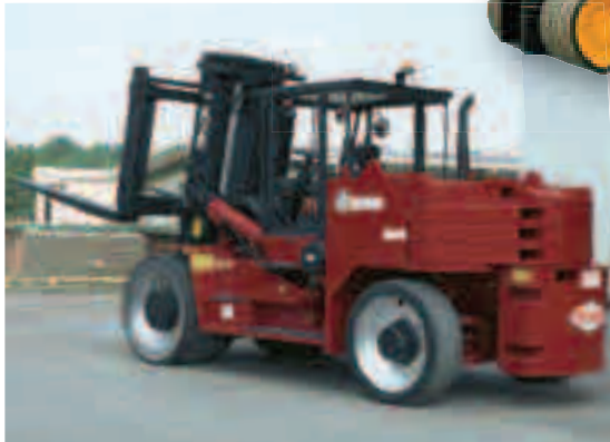
ABOVE: Royal, based in New Century, KS, manufactures a range of specialized rigger trucks. The 80/100 model pictured has a capacity of 80,000 pounds retracted and 100,000 pounds extended at 36 inches
