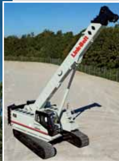
The TCC-450 features a 33 to 105 foot Link-Belt exclusive four section, box boom. It has 11,000 pounds of available line pull from the main winch with 18 mm wire rope. A 197 hp Isuzu engine provides Tier 3 power. Optional equipment includes a rear winch with 11,000 pounds of available line pull and an auxiliary lifting sheave
