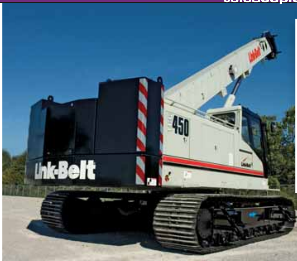
The TCC-450 features a 33 to 105 foot Link-Belt exclusive four section, box boom. It has 11,000 pounds of available line pull from the main winch with 18 mm wire rope. A 197 hp Isuzu engine provides Tier 3 power. Optional equipment includes a rear winch with 11,000 pounds of available line pull and an auxiliary lifting sheave
