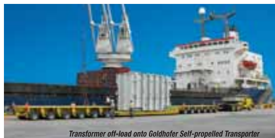
Transformer off-load onto Goldhofer Self-propelled Transporter
