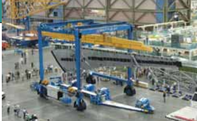
A Shuttlelift ISL70 lifts and transports a wing section of the new Boeing's 787 commercial jetliner
