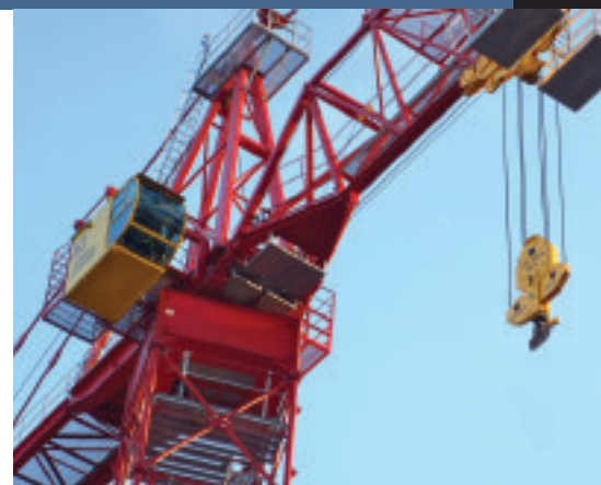
The Kroll K1800 is rigged with 250-feet of jib, has a hook height of 112 feet and is fitted with 176,000 pounds of counterweight
