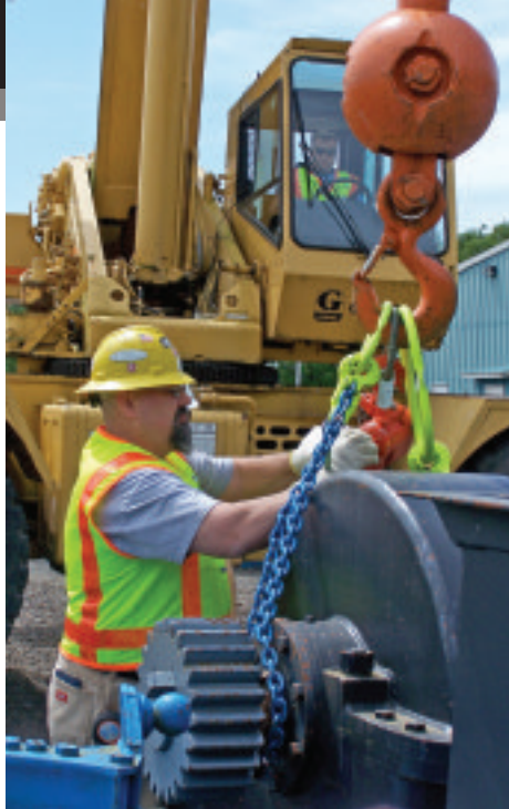
Chain slings are more robust for load corners
