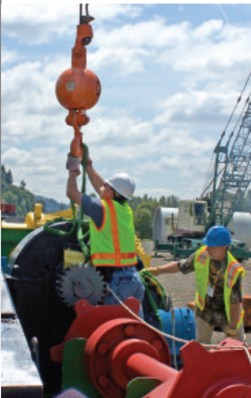
ABOVE: Straightening chain legs helps avoid link damage from twisting
