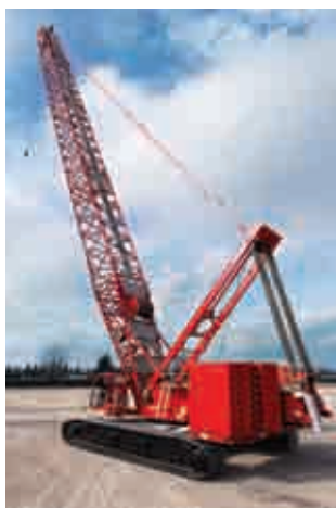
The MLC650 successfully lifted 717 tons of test weights, making the crane's advertised capacity official.
