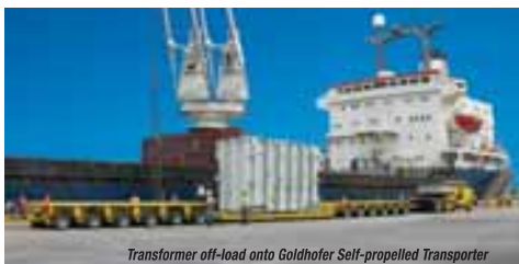
Transformer off-load onto Goldhofer Self-propelled Transporter
