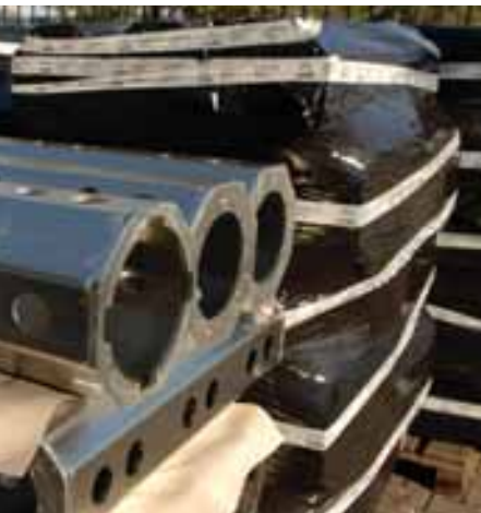
Sections of the tower lifting system at the Hydrospeex factory in the Netherlands prior to shipping to the US. The 1 meter (three foot) long octagonal sections are fabricated from T1 steel on a robotic welding machine
