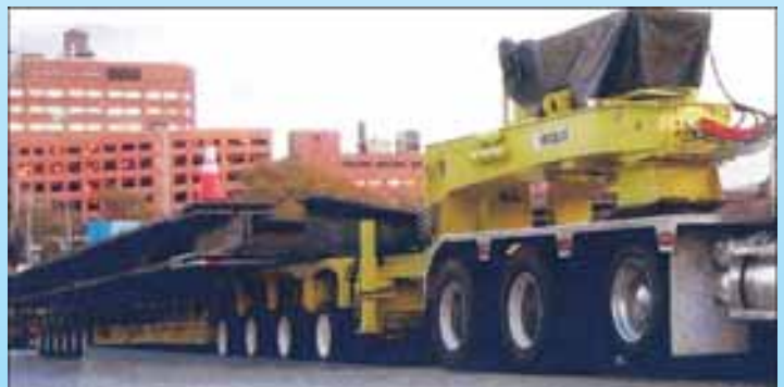
Modules that are used over the road on one job and on site the next. Hauling capacities from 24 to 44 short tons per axle that can be rearranged quickly.
