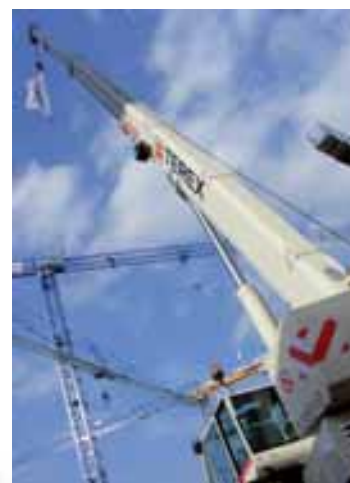
The 34 metric ton capacity RC34 from Terex Bendini
