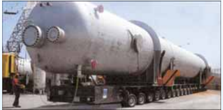
Self propelled modules with 90 degree steering capability for refinery, offshore and industrial applications.
