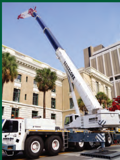
The ATF 400G-6 was rigged with 132 feet of main boom and a 76.9-foot luffing jib at a 40-degree offset.
