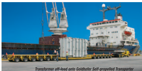
Transformer off-load onto Goldhofer Self-propelled Transporter
