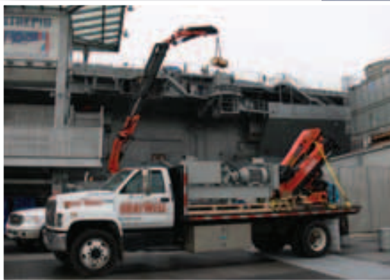
The Palfinger PK 150002G with PJ 170E jib lifts materials to be used for the installation of the smaller Palfinger crane as well as its power unit, shown in the foreground
