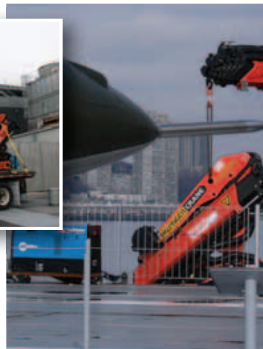
The Palfinger PK 150002G with PJ 170E jib lifts materials to be used for the installation of the smaller Palfinger crane as well as its power unit, shown in the foreground
