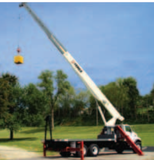
Terex's BT4792 has a lift capacity of 47,000 pounds
