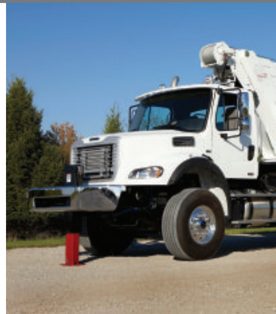
The Elliott 36127F includes a new aluminum bed for reduced weight, a 34-foot 5-inch retracted to 127 foot extended 5-section boom, an internal anti-two block system and a Hirschmann LMI
