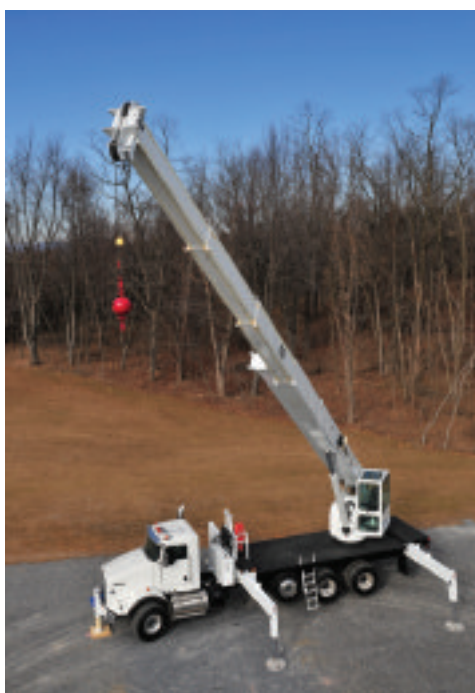
The 38-ton capacity Altec AC38-103S has a 103-foot, 4-section boom
