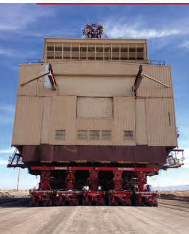
Mammoet moved an 8-million pound Peabody Energy dragline across the New Mexico desert to the El Segundo Mine.
