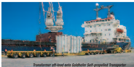
Transformer off-load onto Goldhofer Self-propelled Transporter
