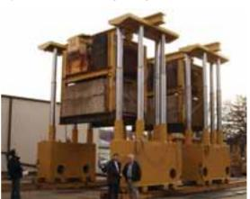
off the system when the load reaches a predetermined height.
