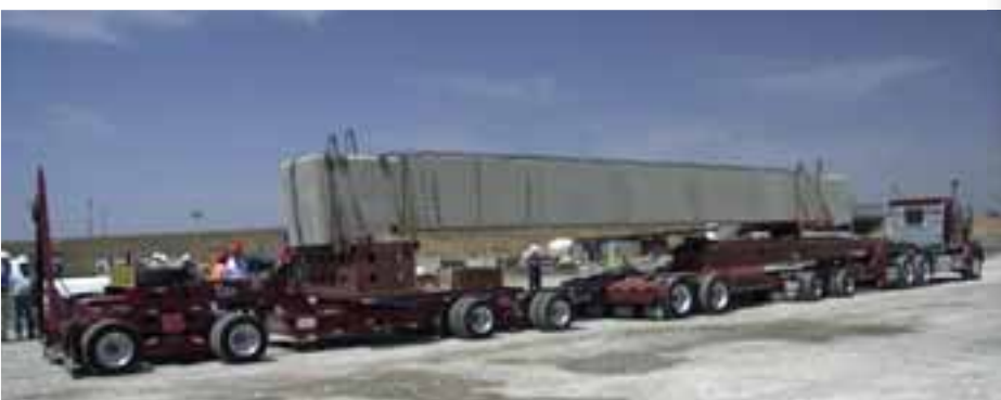
The beam was hauled on an 11 axle unit comprised of a tractor, two jeeps and a steerable dolly
