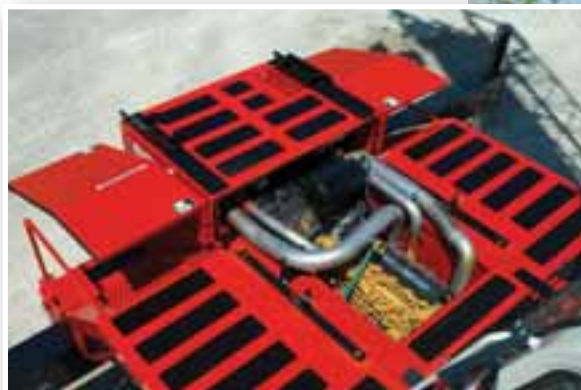
Powering the RTC-8090 Series II is the 225 hp (167.8 kW) Caterpillar C6.6 engine. A direct-mount Spicer powershift transmission takes the power to the wheels. It has six forward and six reverse speeds. A switch in the operator's cab controls the four steering modes: two-wheel front, two-wheel rear, four-wheel, and crab
