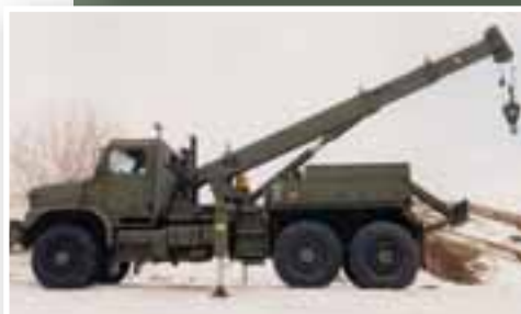
The Marine crane built by Manitex is a 17 tonner with 31 foot boom. It interfaces to OshKosh's hydraulic and remote control system.
