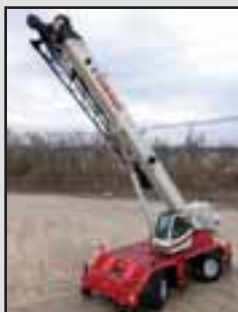
New 2007 RTC-8050II 50 ton Rough terrain crane
