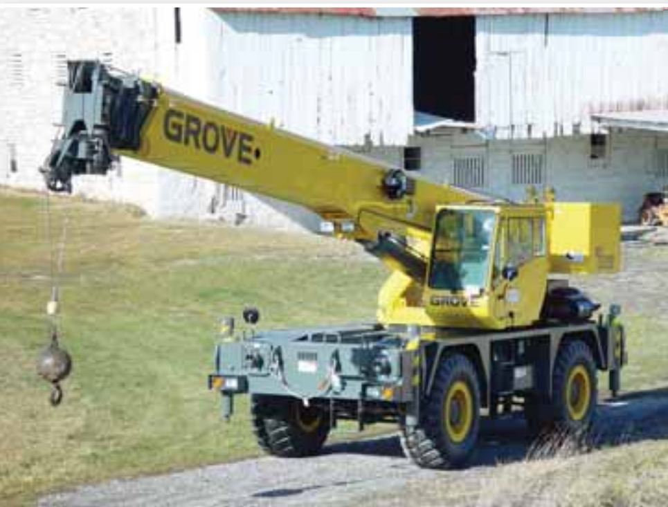
The 35 ton capacity 2007 Grove RT535E features a four-section full power boom and a new crane cab with improved instrumentation and control panel inside
