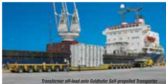
Transformer off-load onto Goldhofer Self-propelled Transporter
