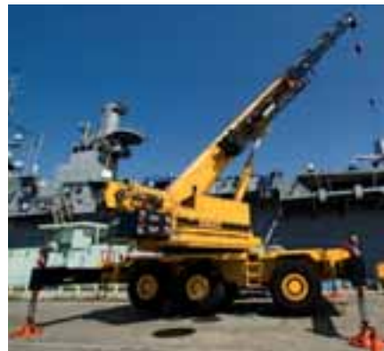
An RTC-80100 Series II Link-Belt hoists a load onto an aircraft carrier
