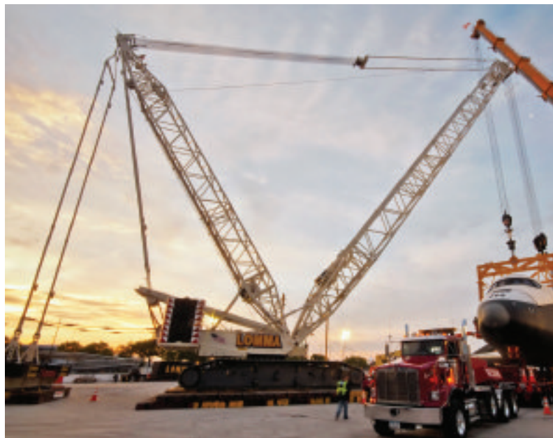
A Terex CC 2800-1 crawler crane was recently used to lift the Space Shuttles Discovery and Enterprise
