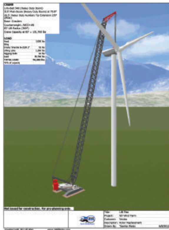
A wind turbine lift plan is demonstrated using a Link-Belt 548 crawler
