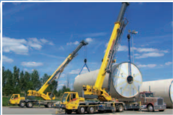
Twin Grove TMS800E models owned by W.D. Grubb lift 36 ton storage vats at the Port of Richmond in Virginia. The vats were transported to a Coors Brewery
