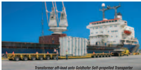
Transformer off-load onto Goldhofer Self-propelled Transporter
