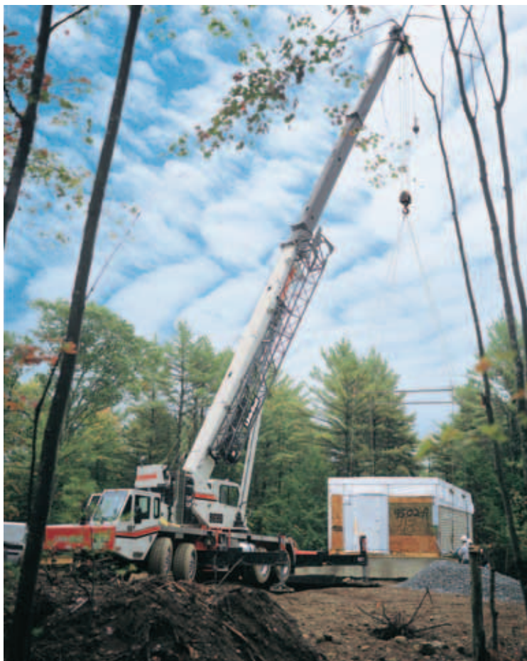
With a 90 ton capacity and a five-section 140 foot boom, Link-Belt says its HTC 8690 has found strong acceptance in the higher end of the truck crane market
