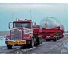
the crews maneuvered onto the McNary Highway to cross back into Washington and pressed on another 200 miles to the project site near Moses Lake. A low bridge on the main highway necessitated a detour onto a series of country roads. Emmert used five 55-foot barge ramps and five 40-foot barge ramps to jump two county bridges with a weight limit of 40 tons. To avoid interference with farm traffic, the permit required the bridges to be fully illuminated and jumped at night.
