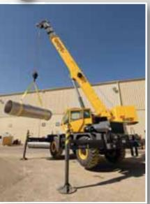
Introduced in 2008 from Manitowoc was the Grove RT540E. The crane features dual-axis, electronic joysticks and a sleeker, more modern cab.
