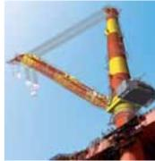
**GERMANY:** The new 2,000 metric ton (2,240 US ton) capacity class MTC 78000 is Liebherr's entry into a new market segment of heavy lift cranes for offshore applications.
