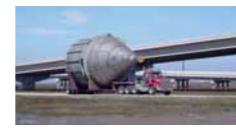
escorts, the load moved safely through all obstacles. Upon arrival at the Shintech docks, the cyclone was positioned by Emmert so that it could be offloaded from the trailer and loaded onto the prearranged configuration on the barge.
