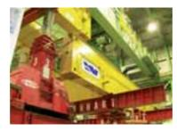
specialized lifting device was fabricated. The device was designed to attach directly into the existing overhead crane hook, effectively eliminating the tight headroom issues. The device allowed Barnhart to enter the crane half through the top, rotate 90 degrees, and attach to the crane half girder flange.
