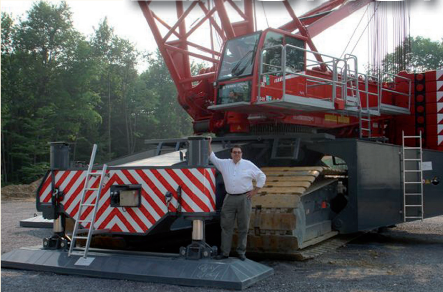
James Lomma in 2007 at a wind farm where his company's narrow track Terex Demag CC 2800 worked setting wind turbines
