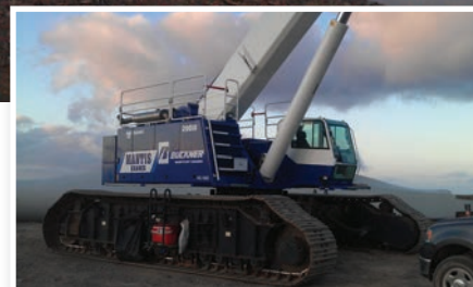
Buckner HeavyLift utilizes its fleet of 100 to 120-ton telecrawlers as assist cranes on wind turbine erection jobsites. Pictured is a 100-ton Mantis telecrawlers working on a wind farm on Maui in Hawaii
