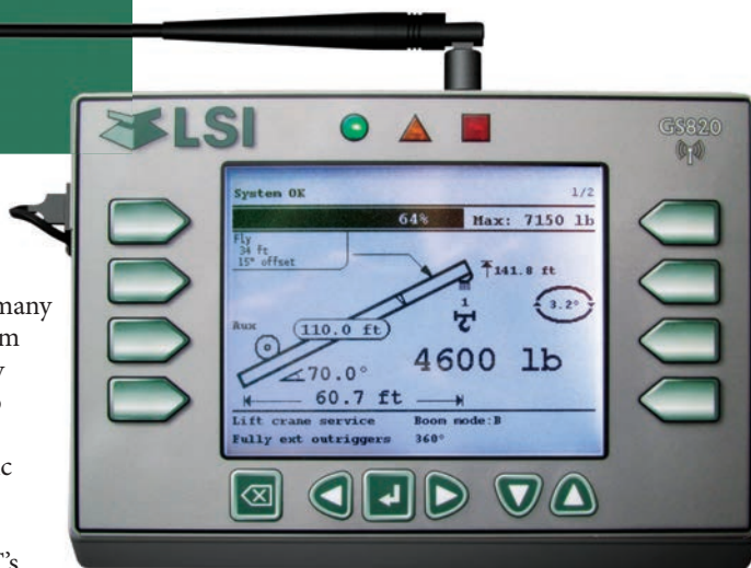
Multi Sensor Graphical Display from Load Systems International. The GS820 monitors any combination of LSI wireless sensor data
