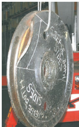
A defense photo shows the crane was two-blocked
