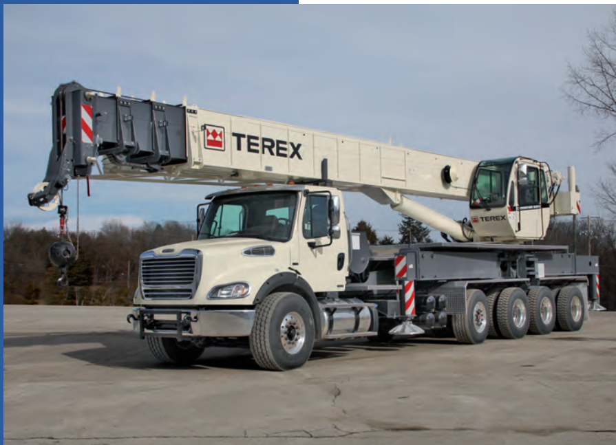
Terex's Crossover 6000 features a 60-ton capacity and uses the upper works from the Terex T560 truck crane.
