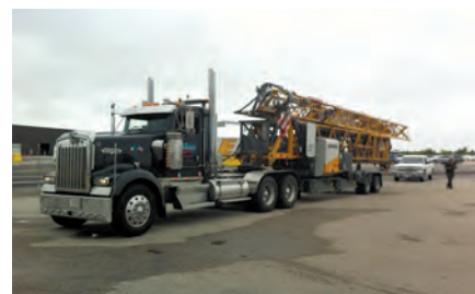
With a packing size of about 7.8 feet by 3.6 feet, the 81 K can be easily transported by boat, truck or rail.
