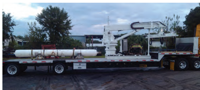
The U.S. Navy target launcher has a boom much like that of a telescopic crane.
