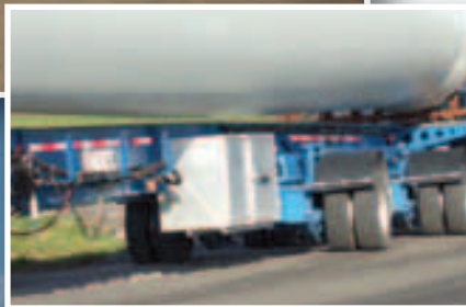
TOP: Burkhalter's driver makes a 90 degree turn using one of its rear steering extendable "blade trailers" in upstate New York INSET: A close-up of the axles while steering in a 90 degree right hand turn
