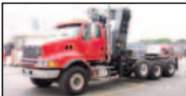
NEW 2005 STERLING TRI/A & 55-TON/M BOOM Knuckle Boom behind cab, fifth wheel and Pusher Axle, 4-stab, 5-ton winch, Radio Remote. Boom handles: 47,000 lb @ 8', 21,000 lb @ 18', 33' hyd. side reach. HEAVY DUTY UNIT - SALE PRICE $169,300
