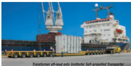
Transformer off-load onto Goldhofer Self-propelled Transporter
