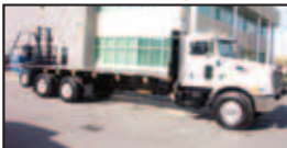
NEW 2006 PETERBILT WITH 3WD PIGGY-BACK New 24' 2" Flat Deck, NEW PRINCETON PBX Double-Reach Piggy-Back, 3WD, 5,000 lb cap. Truck has 330 HP Cummins, 20F/46R on air ride, 8LL. Lots of options. COMPLETE READY TO WORK PACKAGE!
