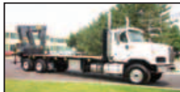
NEW 2006 INTER-L 5600 WITH 70 TON/M BOOM HEILA HLR 70000-3s at rear, front axle stab, 22 ft. deck, RADIO REMOTE. Boom handles: 60,000 lb @ 8', 27,000 lb @ 19', 14,500 lb @ 28'. Heavy-Duty truck, 365 HP, 18 spd. HEAVY PRE-CAST HANDLER
