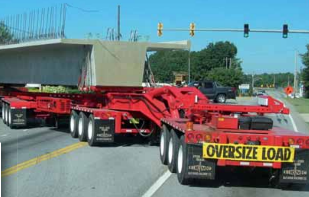
The ERM nine-axle Hydra-Steer trailer with dual steering enhances the load and go skid steer method with new single frame steering capability. The steering improves the versatility during extremely heavy loads and back hauling
