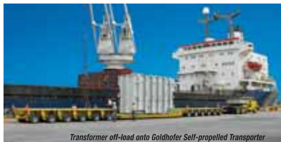
Transformer off-load onto Goldhofer Self-propelled Transporter
