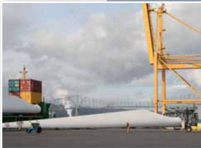
A custom-built transporter and dolly system is used to transport wind turbine blades from the Port of Longview's dock to a temporary storage yard
