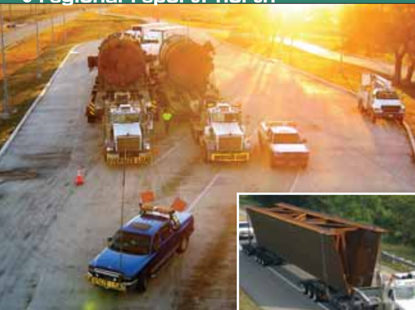
LEFT: A pair of 150 ton reactors moved 3,000 permit miles from Houston, TX to northern Alberta, Canada. As run by Perkins Specialized Transportation Contracting, a pair of tractors were used on each of the dual lane loading trailers to push and pull the loaded transporter. Loaded dimensions were 210 feet long, 18 feet wide, 20 feet high, with a gross vehicle weight of 550,000 pounds
