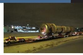
The 155 foot long vessel was transported using a Goldhofer dollied system with the vessel being an integral part of the configuration by holding the two trailers together
