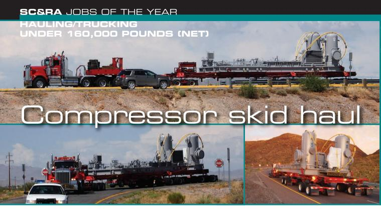
rom April to July, Emmert International, Clackamas, OR, successfully moved seven compressor skids from the plant where they were manufactured in Midland, TX, to the project site in Tupman, CA. Each compressor weighed 140,000 pounds and measured 44 feet, 7 inches long by 19 feet, 4 inches wide by 12 feet, 10 inches tall.
