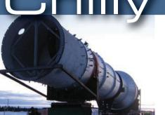
The sulfur reduction unit was transported on a dual Goldhofer 4-file, 10-line trailer configuration. The total gross weight on the highway reached 1.731.519 pounds
