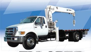
Maximum lifting capacity 10 Ton
