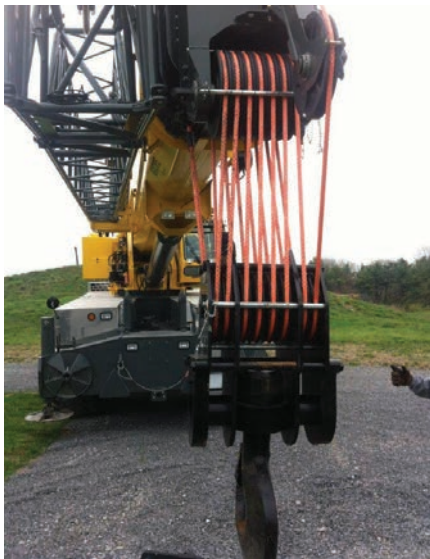
KZ™100 synthetic hoist rope makes its debut on the recently launched Manitowoc RT770E.
