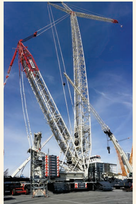
The tallest crane in the history of ConExpo was the Terex Superlift 3800, a 716-ton lattice boom crawler.
