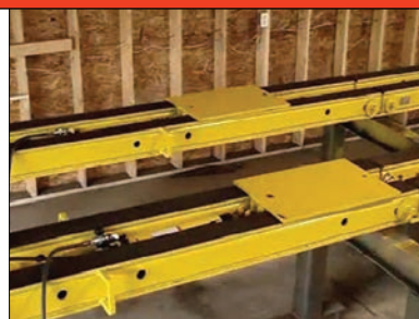
500 Ton Slide System w/ Slide Plates and Push Cylinders
