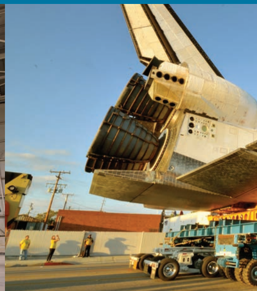
Endeavour is secured to Saren's SPMT system before starting on its 12-mile journey through the streets of Los Angeles
