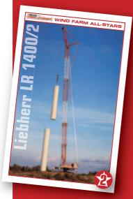
The LR 1400/2 distinguishes itself due its multi-functional boom system, quick crane assembly and cost-effective transport of crane components. The 400 ton machine is controlled and monitored via the LICCONcomputer system. As wind turbines become taller and heavier, the Liebherr LR 1750 will become a heavy hitter in US wind farm work
