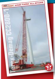
The CC 2800-1 can be converted from being a standard crane into one dedicated to wind power applications by means of a few accessory devices. Fitted with a 90 meter SH/LH SGLmax main boom plus special LF2 12 m (40 foot) wind power jib, the crane hoists loads weighing up to 125 tonnes (138 tons) to a hub height of 94 meters (hook height 102 m) (308 and 335 feet)
