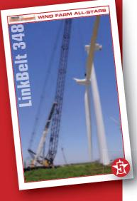
The LinkBelt 348 has the capacity and reach to set the mid and lower sections of wind turbines, and can crawl between foundations with ease
