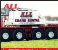
**Grove GMK6300B -** 1998, 300 Ton, Cummins Diesels, 197' Main Boom, 167' Fixed Jib, 200' Luffing Jib, Aux Hoist. **Call Shaune Rados: 216-524-6550**
