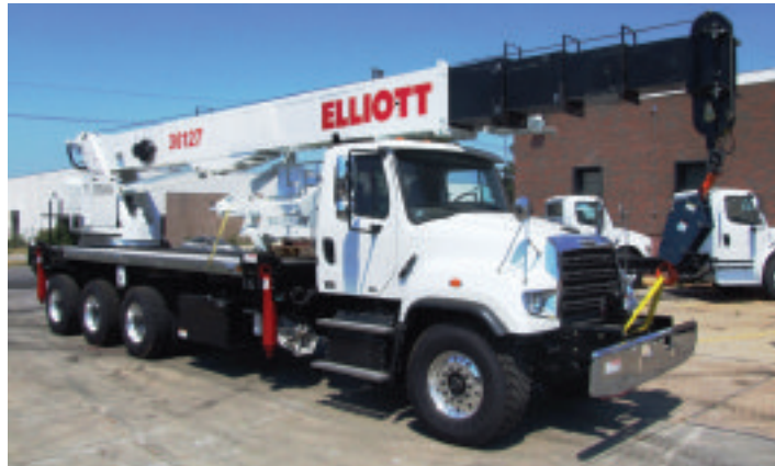
The new 36127R is a 36-ton capacity rear-mounted boom truck
