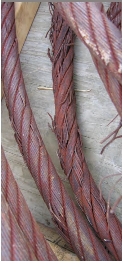
An examination of the failed boom hoist wire rope revealed that the wire rope had gone without the proper lubrication. There were also significant broken wires within the rope strands.
