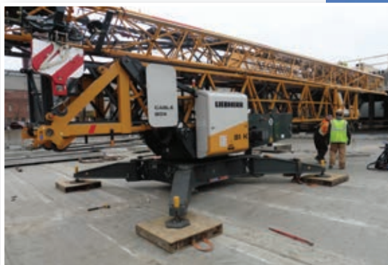
One of Morrow's Liebherr 81 K self-erecting tower cranes is prepared for erection on site in Columbia, MO.
