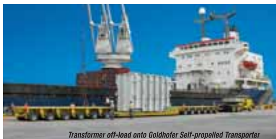
Transformer off-load onto Goldhofer Self-propelled Transporter
