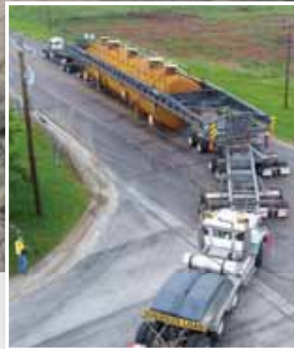
Perkins utilized one of its dual-lane highway transporters with a high girder bridge suspension system
