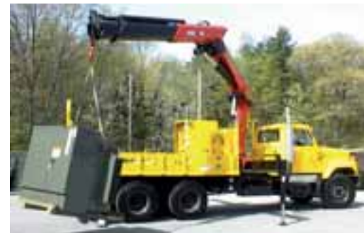
A Palfinger Model 32000 lifting transformers
