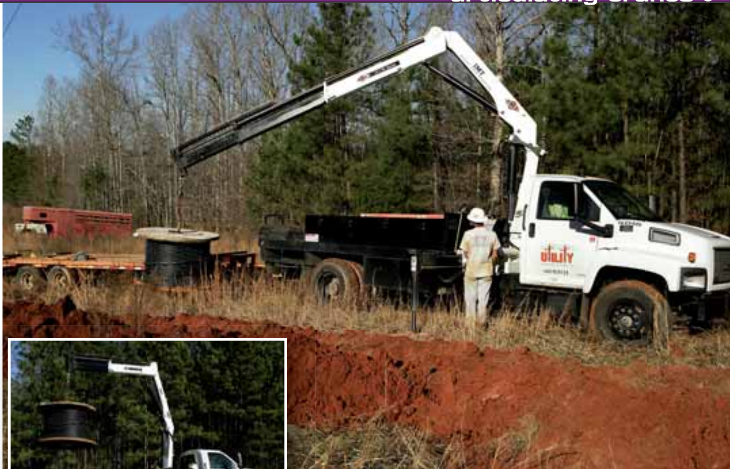
The essential differences between a telescopic crane and an articulating crane are height capacity and payload transportation ability. Iowa Mold Tool has increased its product line to meet demand for this increasingly popular crane
