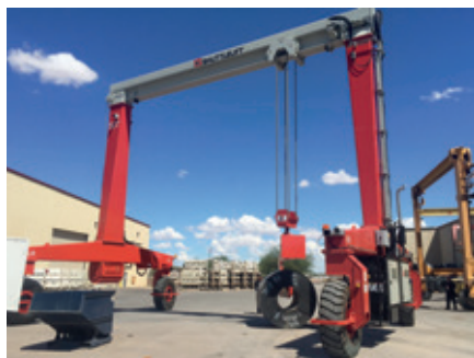
The SB50 gantry crane is the first Shuttlelift to incorporate a unique C hook design to assist with the handling of large steel coils.
