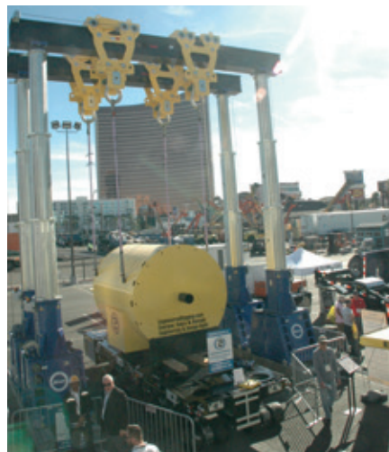
An Enerpac SBL 500 gantry was shown in a lifting configuration with beam and side shift systems.
