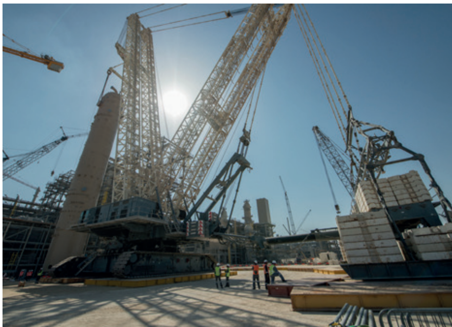
A Demag CC 8800-1 TWIN, with a capacity of 3,200 tons, works at a refinery in Qatar.
