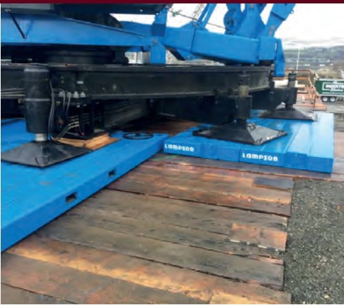
Lampson International uses its steel mats under its Transi-Lift crawler cranes.
