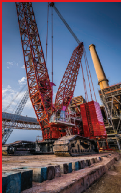
The biggest lift so far has been a 101-ton segment of duct work, which the MLC650 lifted to a height of 211 feet.
