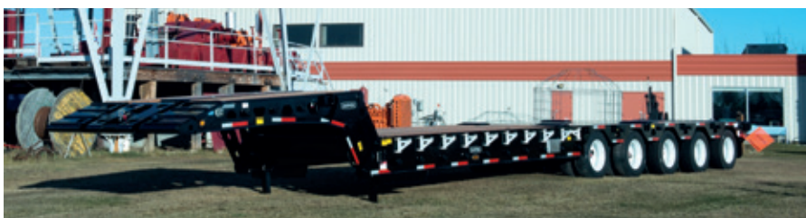
Aspen's Petroleum Series is a line of fixed and folding gooseneck trailers designed for hauling skid-mounted loads.
