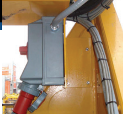
PHOTO 2: Morrow Equipment offers a designated connection box that is separated from the crane's electrical system.
