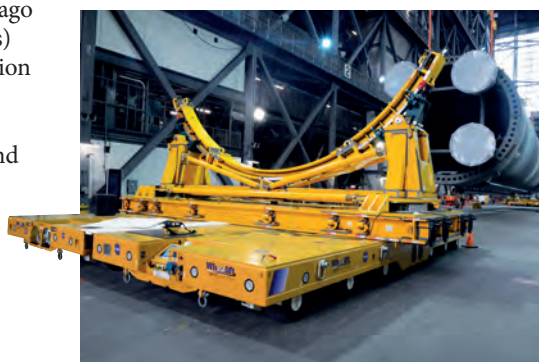
The Aft Lifting Equipment was attached to the rear Colby Crane and tandem-lifted the Core Stage off the transporter.
