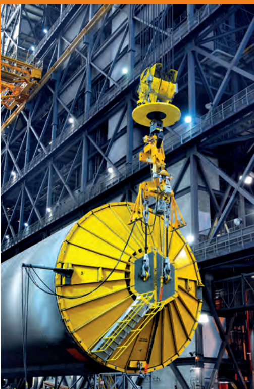
The forward end of the Core Stage Pathfinder was attached to a custom-made spider fixture with leveling capability.
