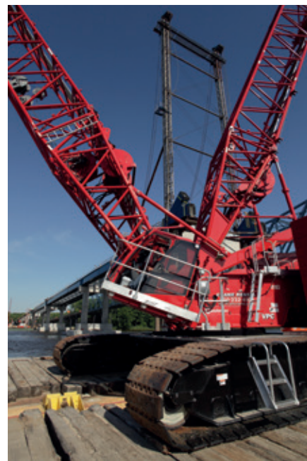
Kraemer North America is using a Manitowoc MLC300 to help replace the 2,482 foot-long Savanna-Sabula Bridge near Savanna, IL. The crane is erected on a 70 by 195-foot a barge in the Mississippi River, and it is lifting 76-ton arch rib sections to a height of 165 feet.
