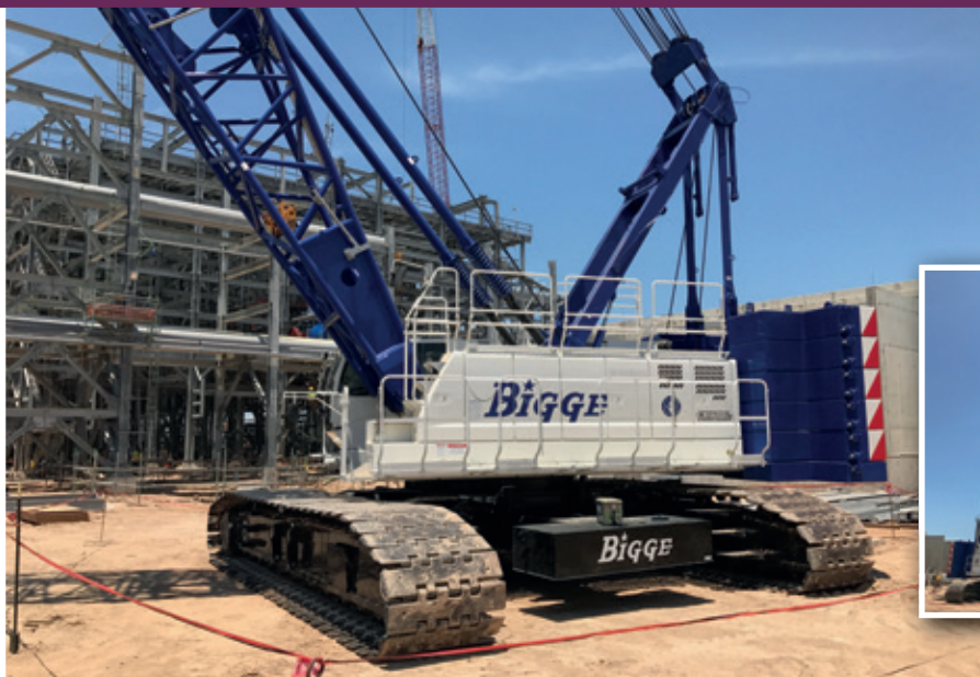
Bigge Crane & Rigging's 160-ton capacity Kobelco CK1600G works at a multi-billion dollar Liquefied Natural Gas Pretreatment facility in Freeport, TX. The crane is erecting steel sections that weigh up to 10,000 pounds each.
