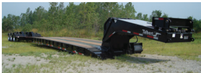
The 55SA-TELE offers strong lift and load heights thanks to the robust, four-cylinder hydraulic removable gooseneck, Talbert said.
