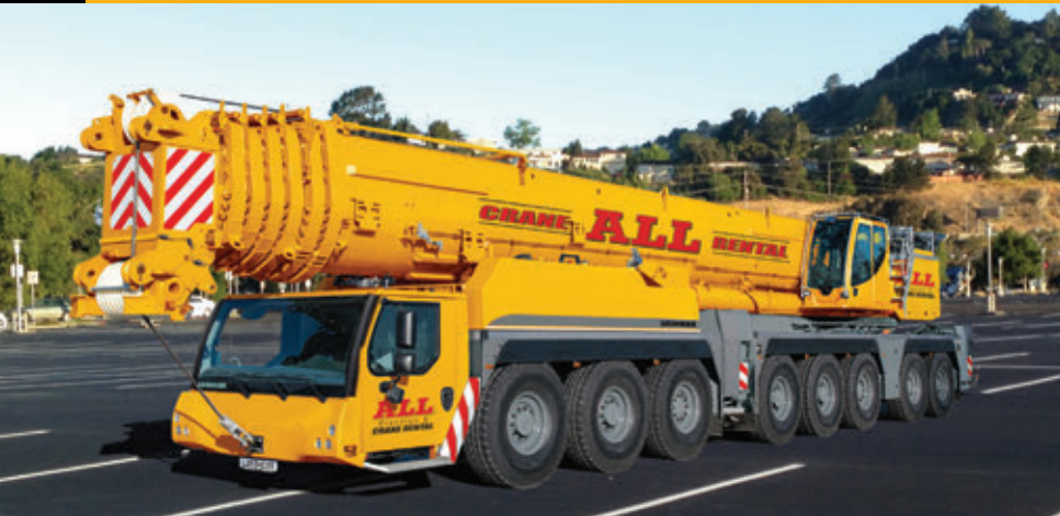
The Liebherr eight-axle LTM 1450-8.1 all terrain crane has a capacity of 500 tons.
