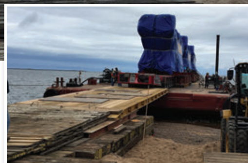
Each of the three engines was unloaded from the barge using a 14-axle line Goldhofer PST-H (self-propelled) and then staged on the frontage road.
