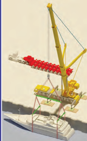
LiftPlanner "Intelligent 3D model" Boat lift
