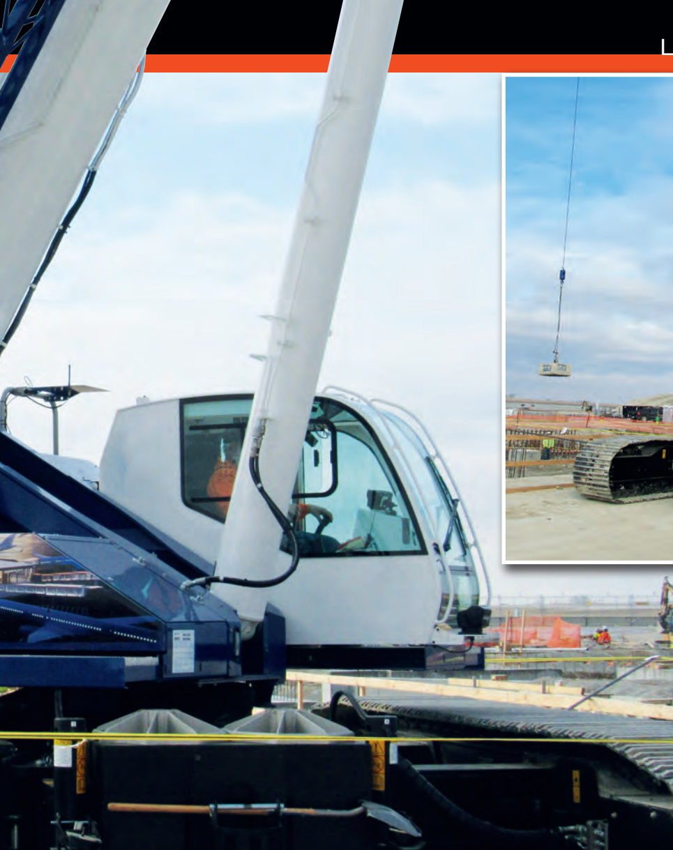
The GTC-800 telescopic crawler delivers 88 tons of “pick & carry” capacity and boasts a max tip height of 198 feet.
