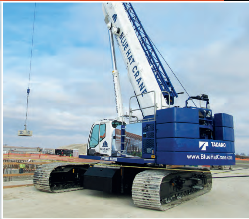
The GTC-800 telescopic crawler delivers 88 tons of “pick & carry” capacity and boasts a max tip height of 198 feet.
