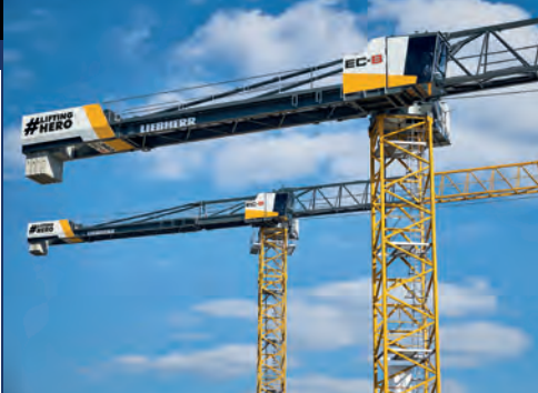
The Liebherr 340 EC-B features synthetic fiber rope.
