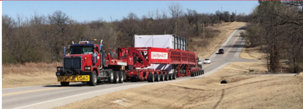
The Barnhart-designed girder system allowed the crew to lift the load up and over a fence to allow the trailer to make it around a corner without civil improvements and without having to remove and replace the fence.
