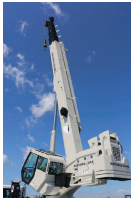
Termed a ‘truck crane replacement,’ the design of the new National NTC55 was influenced by customers who perform taxi crane applications.
