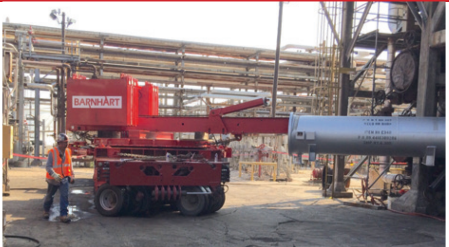
Barnhart's solution involved a custom MOCCS arrangement with 30 kips of counterweight setting atop and secured to a 750-ton hydraulic turntable setting atop and secured to six lines of Goldhofer PSTe. Barnhart named the solution 'The M3A1.'
