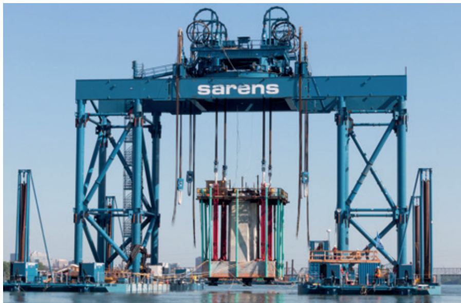
The Sarens' Floating Foundation Installer (FFI) is a self-propelled catamaran that can lift, transport and install foundations.
