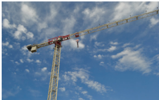
The new CTT 472-20 crane delivers extremely high lift capacities throughout its load chart and 11 different jib configurations from 98.4 to 262.5 feet to meet varying jobsite needs.
