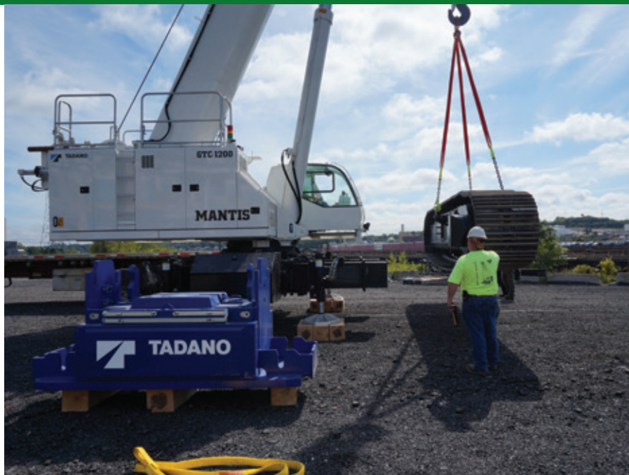
The GTC1200 is a 130-ton crane and has the strongest barge chart of all hydraulic boom crawler cranes.
