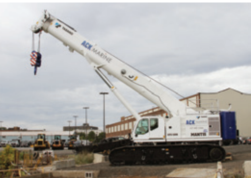
The GTC1200 is a 130-ton crane and has the strongest barge chart of all hydraulic boom crawler cranes.
