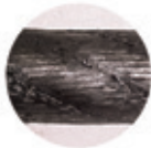
Heavily lubricated rope making inspection difficult
