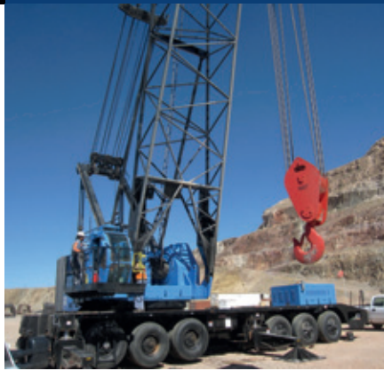
Two years ago WHECO restored a 300-ton conventional truck crane that would have cost millions of dollars to replace.
