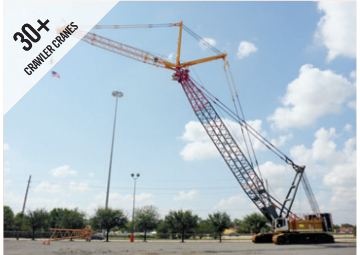
Liebherr LR1250 250 Ton Self Erecting | Houston
