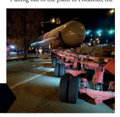
PERMITTED WIDTH/HEIGHT: 20 feet wide, 19 feet 3 inches tall with axle loadings of 42,400 pounds per line ROUTE: 730 miles **MAN HOURS: 7.242** EQUIPMENT USED: 2X Goldhofer THP/CA 11-line dual lane trailers | 6 and 7-foot wide dollies | transport saddles
