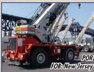
2000 Link-Belt RTC 8030 30-ton, 91' boom, 27' jib. POR
