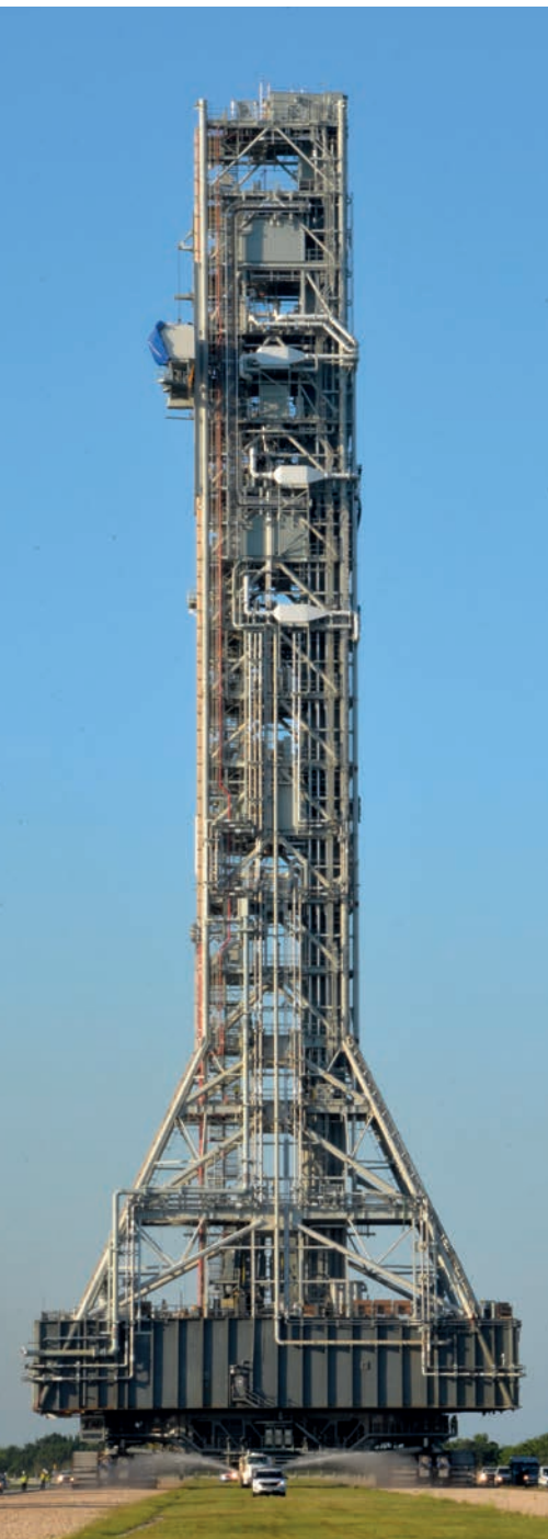
The NASA Crawler-Transporter's height varies from 20 to 26 feet depending on the position of the jacking, equalization and leveling cylinders that work to keep the load level.
