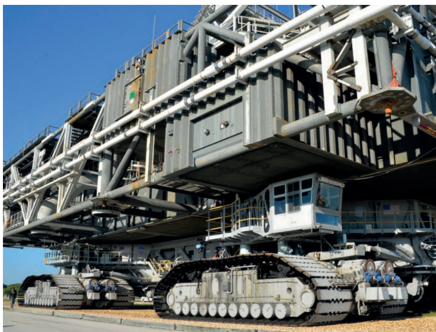
The NASA Crawler-Transporter's height varies from 20 to 26 feet depending on the position of the jacking, equalization and leveling cylinders that work to keep the load level.
