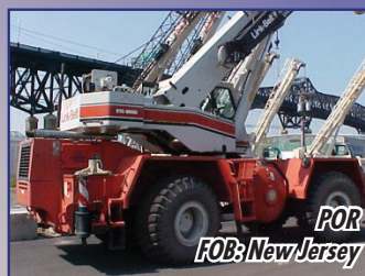
1998 Link-Belt RTC 8035 35 ton, S/N: F118-8006, 91' boom, 25' fly
