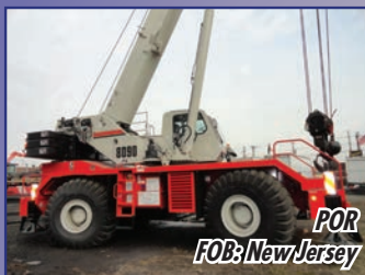
2009 Link-Belt RTC 8090 90 ton, 140' main boom, Aux winch, 35' - 58' 2 pc jib, block-ball. Cat C6.6 diesel
