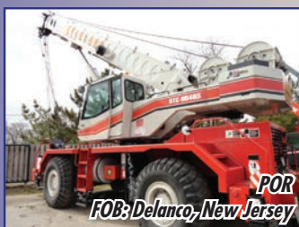
2001 Link-Belt RTC 8040 SII 40-ton, S/N: F7J1-5291, 105' main boom, 28'-51' 2-piece jib, Hydro gas ride, Aux winch, Rear steer indicator
