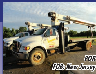
2005 Manitex 1770C 17-Ton, Ford F750 210 HP CAT, 20' wood deck, 23' 1-piece jib
