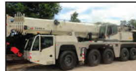
170 TON - TEREX DEMAG AC140 Year: 2012 - 197' Boom / 57' Jib, Dliamler, 2 winches, LMI, Anti-2-Block, Block & Ball
