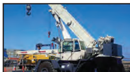
55 TON - TEREX RT555-1 Year: 2012 - Engine: Cummins/Diesel Extras: 2 Winches, LMI, Anti-2-Block, 4x4, Joystick Controls, Block & Ball
