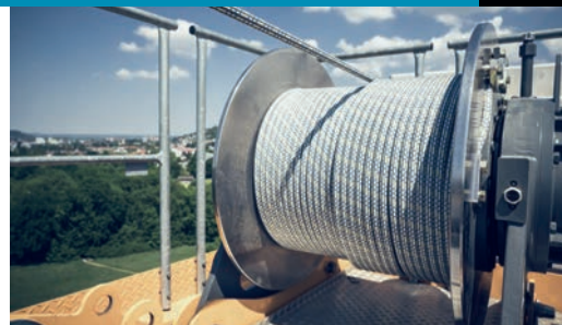
The fiber ropes developed by Liebherr and Teufelberger are being tested in the field.
