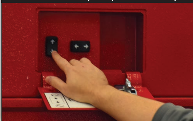
Ground accessible switches for fly assist cylinder and boom hoist cylinder
